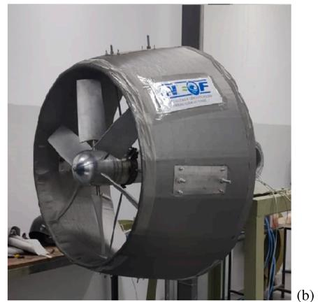
Fig. 17. (a) HDAT Performance and (b) prototype.
